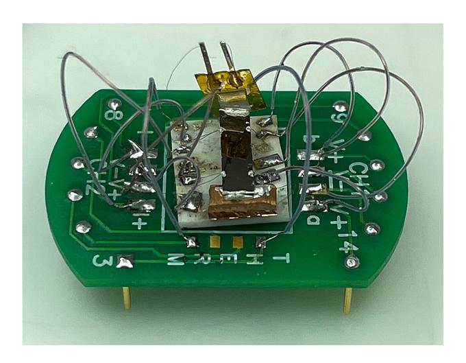
This device tests the properties of the cadmium arsenide thin film—the black strip in the center. Credit: UC Santa Barbara
