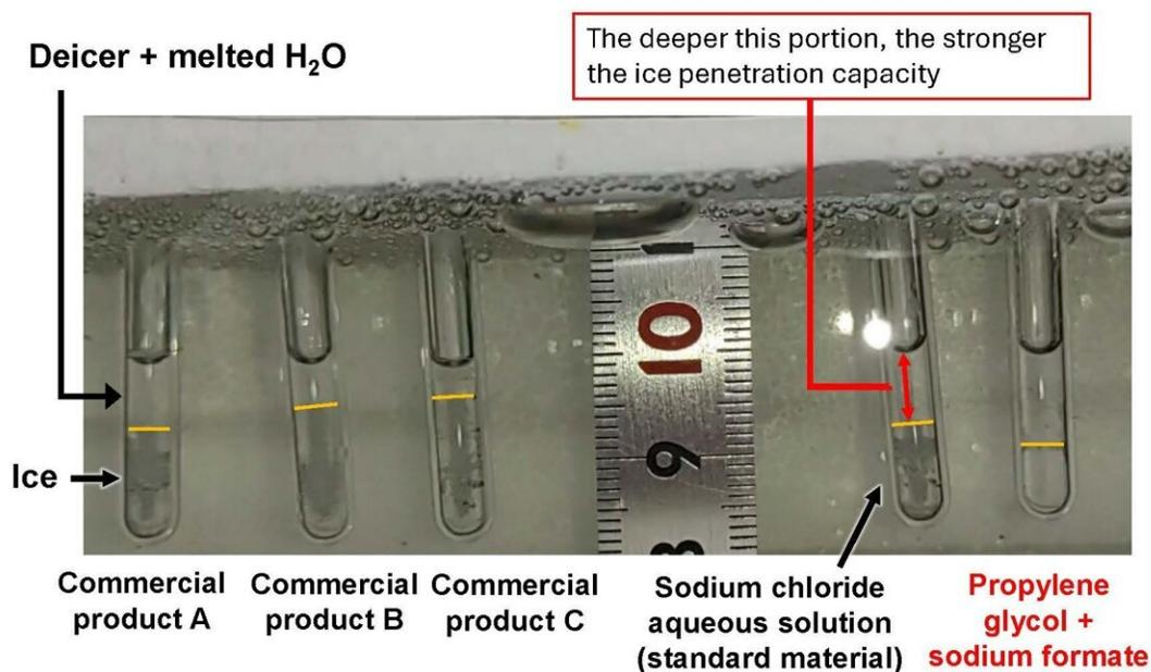
The experiment compared several commercial deicers with an aqueous sodium chloride solution as the control and a new propylene glycol-sodium formate mixture. Credit: Osaka Metropolitan University
