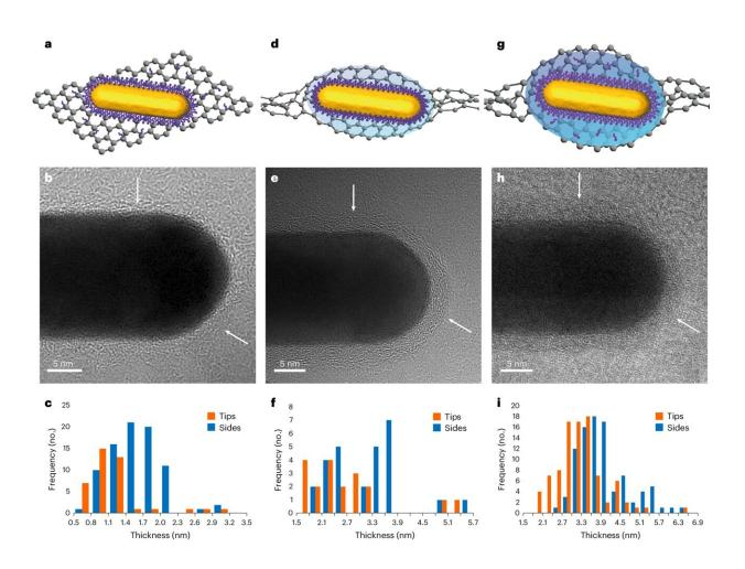
Comparison of TEM investigation of gold NRs capped with CTAB ligands in dried state on a graphene grid and in a liquid environment. Credit: *Nature Chemistry* (2024). DOI: 10.1038/s41557-024-01574-1
