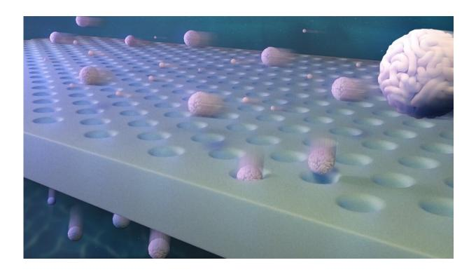
Nanoscale solutes with only slight differences in size can be separated by membranes with identical pores — if they have enough opportunities to try. Credit: Argonne National Laboratory.
