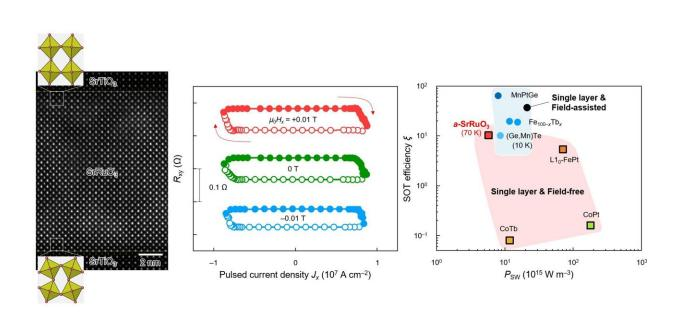
Atomic structure of asymmetric SrRuO<sub>3</sub> thin films and spin-orbit torque magnetization switching results controlled at the atomic layer level. Credit: POSTECH
