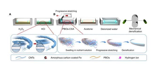
Schematic diagram for fabricating highly packed and aligned fibers. (A) Schematic diagram of functionalization and purification of pristine carbon nanotube fibers (CNTFs). (B) Schematic diagram of the progressive stretching and densification treatment for the highly packed and aligned fibers. Credit: *Science* (2024). DOI: 10.1126/science.adj1082
