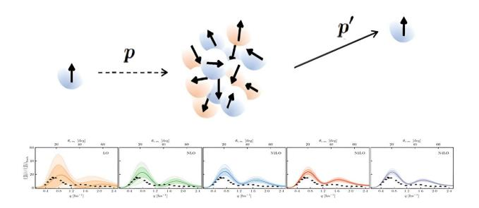
Top: protons striking a nucleus deflect from their original path depending on velocity, location of impact, and force from the protons inside the nucleus. Bottom: elastic proton scattering cross sections from oxygen-16 at different orders of magnitude. Credit: Charlotte Elster
