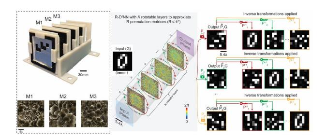
Multiplexed all-optical permutation operations using a reconfigurable diffractive optical network. Credit: UCLA Engineering Institute for Technology Advancement
