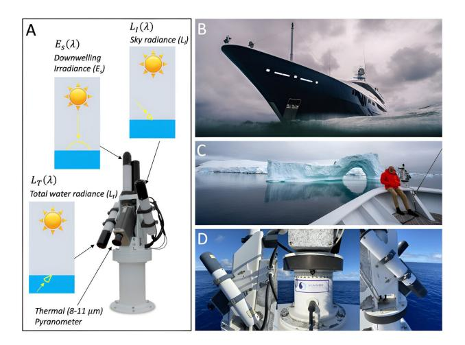
Sea-Bird Scientific Solar Tracker Aiming System measuring total water radiance and sky radiance at a solid angle, and downwelling irradiance, which are used to compute remote sensing reflectance. Reproduced with permission from Sea-Bird Scientific (2017). Credit: *Frontiers in Remote Sensing* (2024). DOI: 10.3389/frsen.2024.1336494
