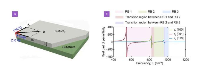
(a) Schematic of  $\alpha$ -MoO<sub>3</sub>/substrate heterostructure, where the substrate is SiC or Au. (b) Real parts of the components of the dielectric tensor of  $\alpha$ -MoO<sub>3</sub> along the principal directions. The Reststrahlen bands are shaded in different colors. Credit: *Opto-Electronic Science* (2024). DOI: 10.29026/oes.2024.240002
