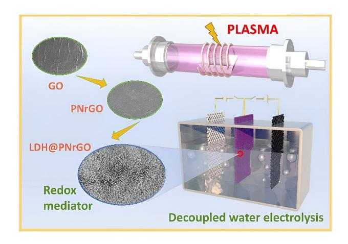
Plasma-assisted preparation of high-capacity bipolar electrodes for hydrogen production by two-step water electrolysis. Credit: Chen Changlun
