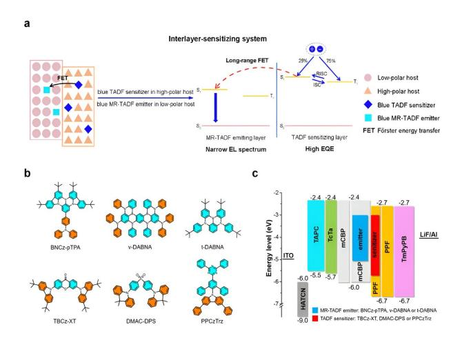
a, Schematic illustrations of interlayer-sensitizing system for blue MR-TADF emitters. b, Molecular structures of MR-TADF emitters and TADF sensitizers employed in the interlayer-sensitizing configuration. c, Device configuration of interlayer-sensitized hyperfluorescence devices. Credit: Jianghui Wang, Peng Zou, Letian Chen, Zhentao Bai, Hao Liu, Wen-Cheng Chen, Yanping Huo, Ben
