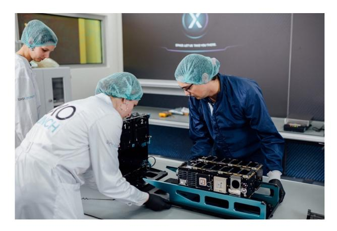
CURIE team members work on integrating the satellites into the CubeSat deployer. Credit: ExoLaunch
