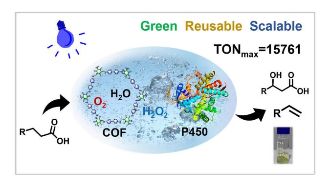
An artificial photoenzymatic cascade was built through combining the photocatalytic  $H_2O_2$  production by COF-TfpBpy with the  $H_2O_2$ -dependent enzymatic activity of P450 peroxygenases, achieving efficient sacrificial reagent free synthesis of 1-alkenes and hydroxyl fatty acids from naturally abundant fatty acids with only water, air and visible light. Credit: Science China Press
