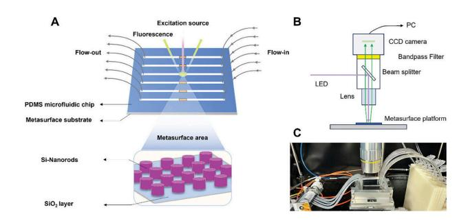
A) Schematic diagram of metasurface platform. Inset figure magnifies the nanostructure of metasurface area; B) The schematic diagram of fluorescence (FL) setup for imaging; C) Actual photograph of experimental configuration for human serum albumin (HSA) detection. Credit: *Advanced Optical Materials* (2024). DOI: 10.1002/adom.202400868
