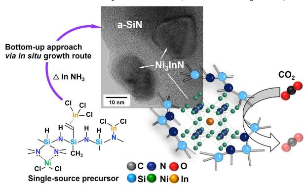
This illustration depicts a novel bottom-up approach developed to synthesize a nanometer-sized Ni<sub>3</sub>InN anti-perovskite/amorphous silicon nitride (a-SiN) nanocomposite via an *in situ* growth route, as well as its unique CO<sub>2</sub> adsorption–desorption properties as a potential small-molecule activation catalyst. Credit: Yuji Iwamoto, Nagoya Institute of Technology
