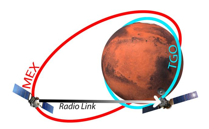
Orbital configuration of Mars express (red) and trace gas orbiter (blue) during a typical mutual radio occultation observation, with a black/white arrow indicating the direction of the radio link between the two spacecraft. Credit: *Radio Science* (2024). DOI: 10.1029/2023RS007873
