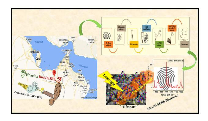
The newly developed label free silver nanoparticle SERS sensor capable of detecting DNA of GJB2 genes causing hearing loss. Credit: 10.1016/j.ijbiomac.2024.129381
