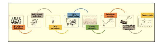
Scheme of real time sensing of deafness mutations with SNA/Si SERS biosensor. Credit: 10.1016/j.ijbiomac.2024.129381
