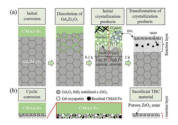
The changes in crystalline products and microstructure of the  $Gd_2Zr_2O_7$  coating with corrosion time and Fe content under CMAS-Fe corrosion are illustrated in a. Meanwhile, b presents the growth mechanism of the reactive layer during CMAS-Fe cyclic corrosion. Credit: *Journal of Advanced Ceramics*, Tsinghua University Press
