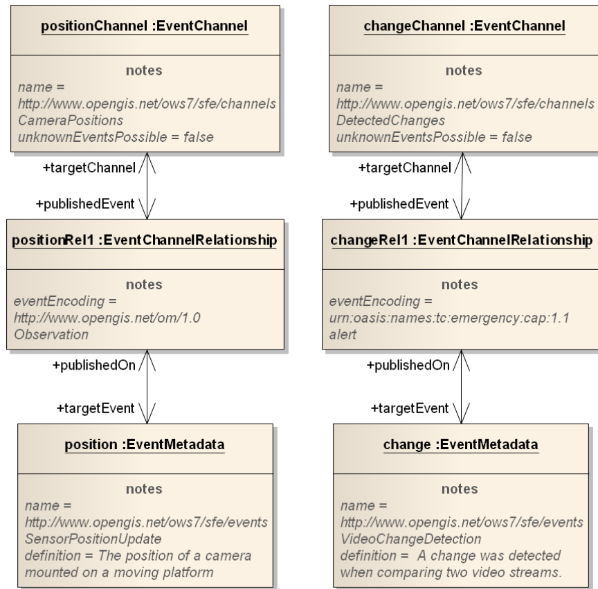
Figure 31: Example of Event Metadata for SFE Service – UML Object Diagram Notation
