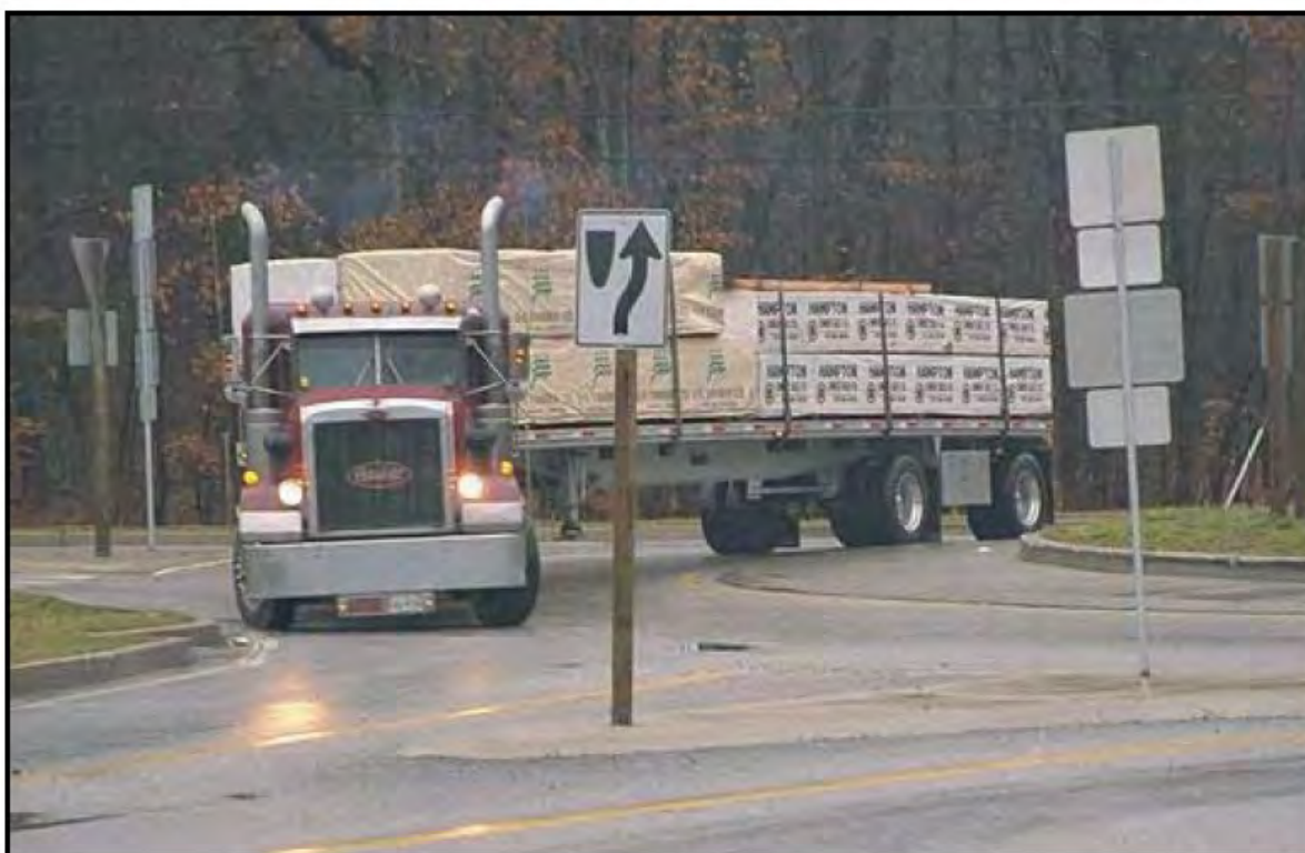
LARGE TRUCK OVERTOPPING THE TRUCK APRON
