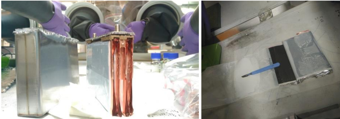
Figure 14: Left - Components of a fresh LMO-NMC/graphite cell after opening and removal of the cell casing in a glove box. Right - Unfolding of one of the two prismatic jelly rolls.
