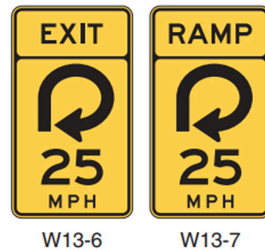
Figure 2. Illustration. Combination Horizontal Alignment/Advisory Exit and Ramp Speed signs (FHWA 2009).
