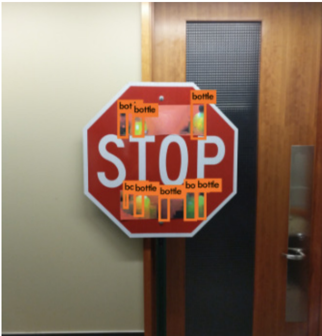
University of Michigan Ph.D. candidate Kevin Eyholt and a team of researchers demonstrate how the strategic placement of stickers on a STOP sign can distort machine perception. Known as physical adversarial perturbation, this tactic can cause inaccurate or missed object classifications, leading to real-world harm (e.g. an autonomous vehicle algorithm not recognizing a STOP sign). (Kevin Eyholt, et al./University of Michigan)
