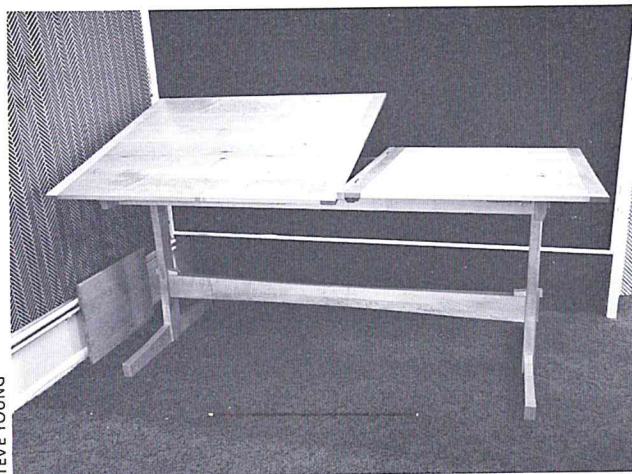
Knockdown writing table. The table, in keeping with Erpelding's style, knocks down, the connecting joints being secured with wedges. The left half of the top can be raised in increments to 45 degrees. The right half lifts to reveal a storage compartment.
