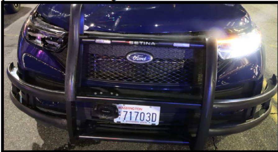
Top: Overview of push bar and damage. Right: Rubber covering after the collision
