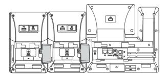
**1.** Connect the USB jack on the host phone and the mini USB jack on the expansion module using one supplied cable.
