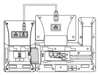
**Note:** Power is automatically transferred from the host phone to the expansion module(s) upon connection. If you want to use more than one expansion modules on a single phone, you need to connect an additional Yealink power adapter (5V/2A) to any one of the expansion modules
