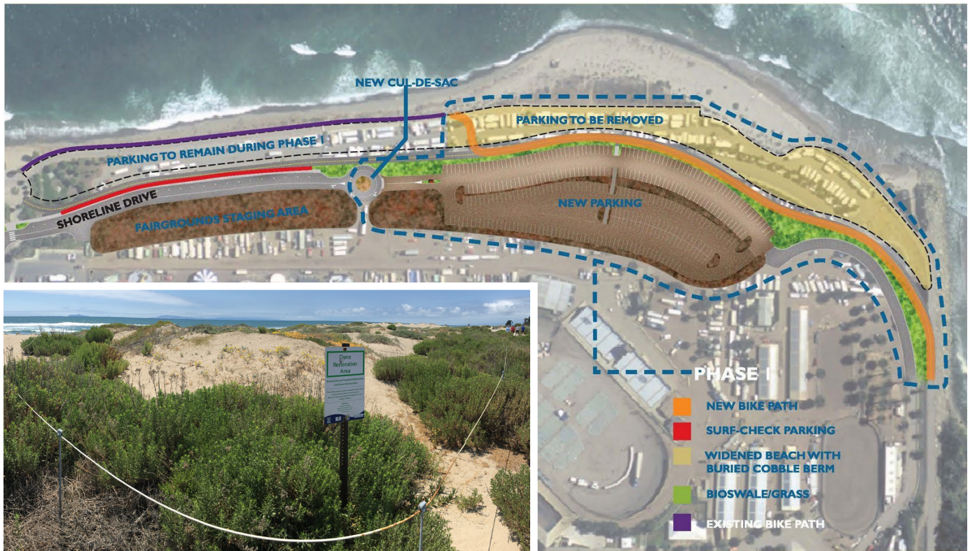
▲ Figure 11: A schematic showing the revised design to accommodate phasing due to budget constraints. Phase 1 (blue dashed lines) was constructed 2010-2012. The remainder of the project, called Phase 2 (highlighted shore areas to the left of Phase 1), has not been constructed. 2009. Image credit: City of Ventura, RRM and PWA. Inset Photo: Restored vegetated dunes in the area labeled as 'parking to be removed' in the design schematic. Photo credit: Paul Jenkin.
