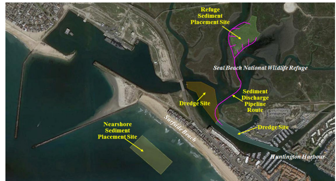
▲ Figure 4: Pipeline route from dredge site to augmentation site at the Refuge. The Nearshore Sediment Placement site was used in the larger dredging project and not the Seal Beach project.
