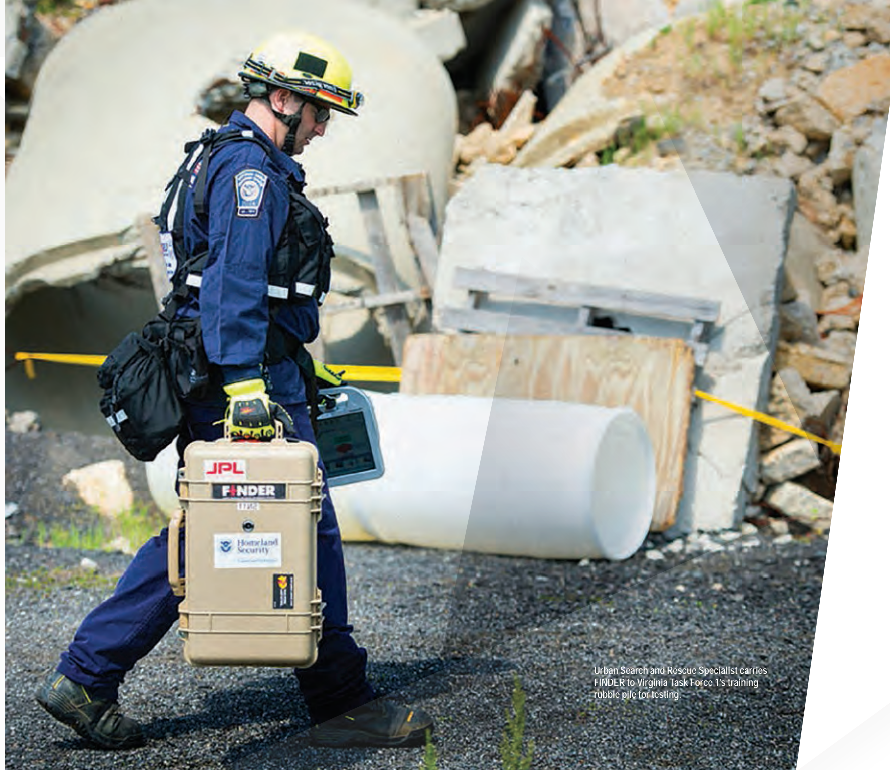
[A] USAID Search and Rescue Team USA-1 prepares FINDER for use in Kathmandu. [B] The NASA/JPL developed FINDER is a portable radar that detects buried victim heartbeat and respiration. [C] Rescuers assist a victim after the Nepal earthquake in April 2015. [Photo credit: EPA Narendra Shrestha].
