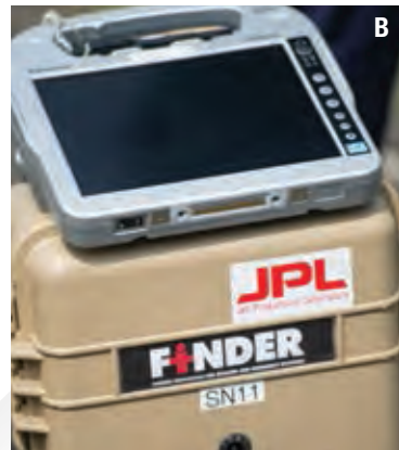
[A] USAID Search and Rescue Team USA-1 prepares FINDER for use in Kathmandu. [B] The NASA/JPL developed FINDER is a portable radar that detects buried victim heartbeat and respiration. [C] Rescuers assist a victim after the Nepal earthquake in April 2015. [Photo credit: EPA Narendra Shrestha].
