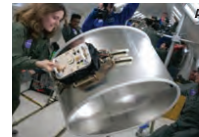
[top left] Principal Investigator Aaron Parness of NASA's JPL and the Stanford University team flew several gecko adhesive based experiments on NASA's zero gravity aircraft during the Aug 2015 campaign. [top center] JPL researchers were inspired by gecko feet, such as the one shown here, in designing a gripping system for space. Just as a gecko's foot has tiny adhesive hairs, the JPL devices have small structures that work in similar ways. [image credit: Wikimedia Commons] [A] Team member Christine Fuller is grappling a free-floating 1-meter diameter aluminum cylinder with a gecko-adhesive enabled gripper. [B] Microscopic image of gecko-like material fabricated in the Microdevices Lab. [C] This artist's concept shows how a future robot called LEMUR (Limbed Excursion Mechanical Utility Robot) could inspect and maintain installations on the International Space Station. The robot would stick to the outside using a gecko-inspired gripping system.
