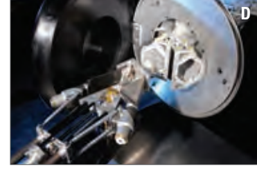
[A] Sampling process: approach, contact, sample, retract [right to left]. [B] Sampling chain testbed. [C] A void is left in the simulant where the sample was acquired. [D] A lid retains the sample in a Sample Return Capsule chamber. [left] Principal Investigator Paul Backes in the sampling chain testbed.
