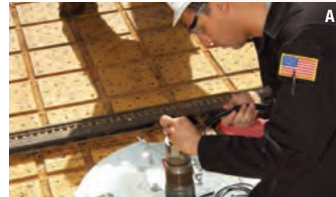
A Deep Exploration Biosphere Investigative tool team deploying DEBI-t into a borehole 0.5 km below ocean floor for in-situ microbial analysis.
