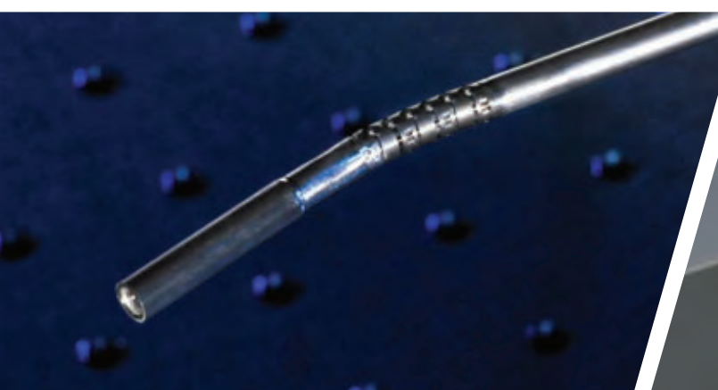
[top] This technology will allow surgeons to perform procedures quicker, safer and more precisely, resulting in better outcomes and lower costs for both hospitals and patients. [above] A tiny, electronic, high-definition 3-D camera mounted on the tip of the endoscope. [right] Laboratory prototype of MARVEL, one of the world's smallest, steerable 3-D cameras.
