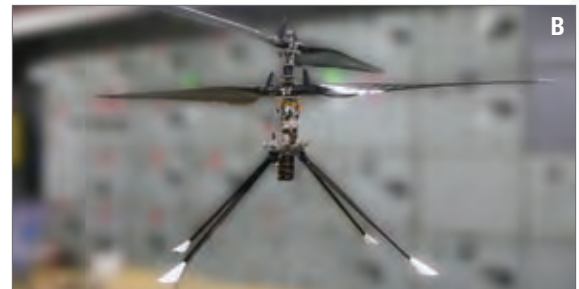
[A] The Mars helicopter would help scout for areas of highest scientific interest and choose the safest and fastest route to get there. [B] Prototype Mars helicopter has a 1.2-meter tip-to-tip diameter rotor system and weighs about 1.4 kg.
