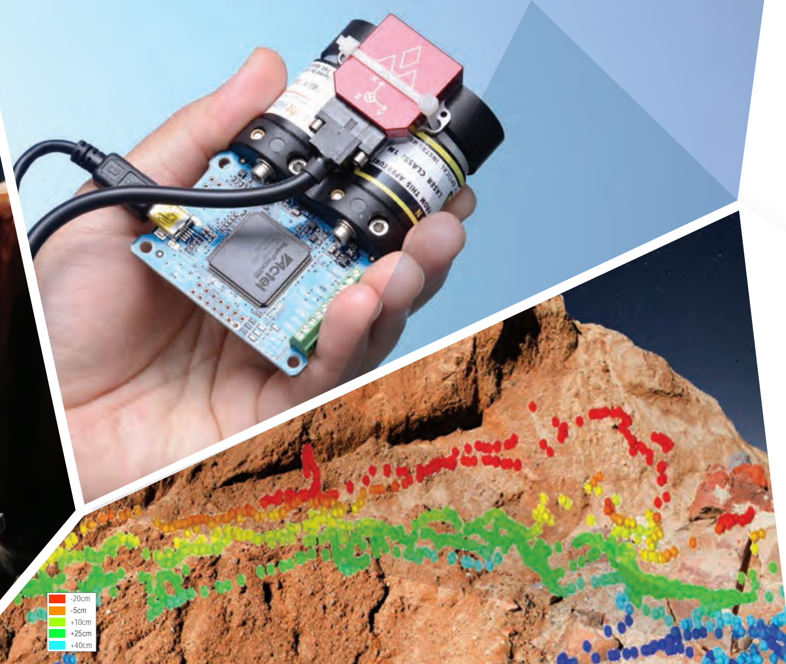
[top] Commercial low-cost CMOS inertial measurement unit (IMU) developed for gaming platforms — can track their own orientation (theta, phi) — is coupled to a low cost CMOS LIDAR system to measure range. [above] Shown is a JPL Mars yard demonstration of collected laser range (LIDAR) measurements using a CMOS IMU. The IMU orientation data would be used to create a map and be combined with data from other remote sensors such as terahertz detectors, Hyperspectral imagers, and LIDAR — without the need of a scan platform.
