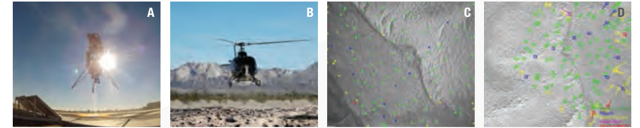
[A] Testing of the LVS payload on the Autonomous Descent and Ascent Powered-flight Testbed, in-flight at Mojave, CA. [B] LVS helicopter field testing over Mars-analog terrains. [C-D] LVS correlates camera images collected in flight (left) against a pre-stored map (right) to accurately determine the vehicle position, attitude, and velocity.
