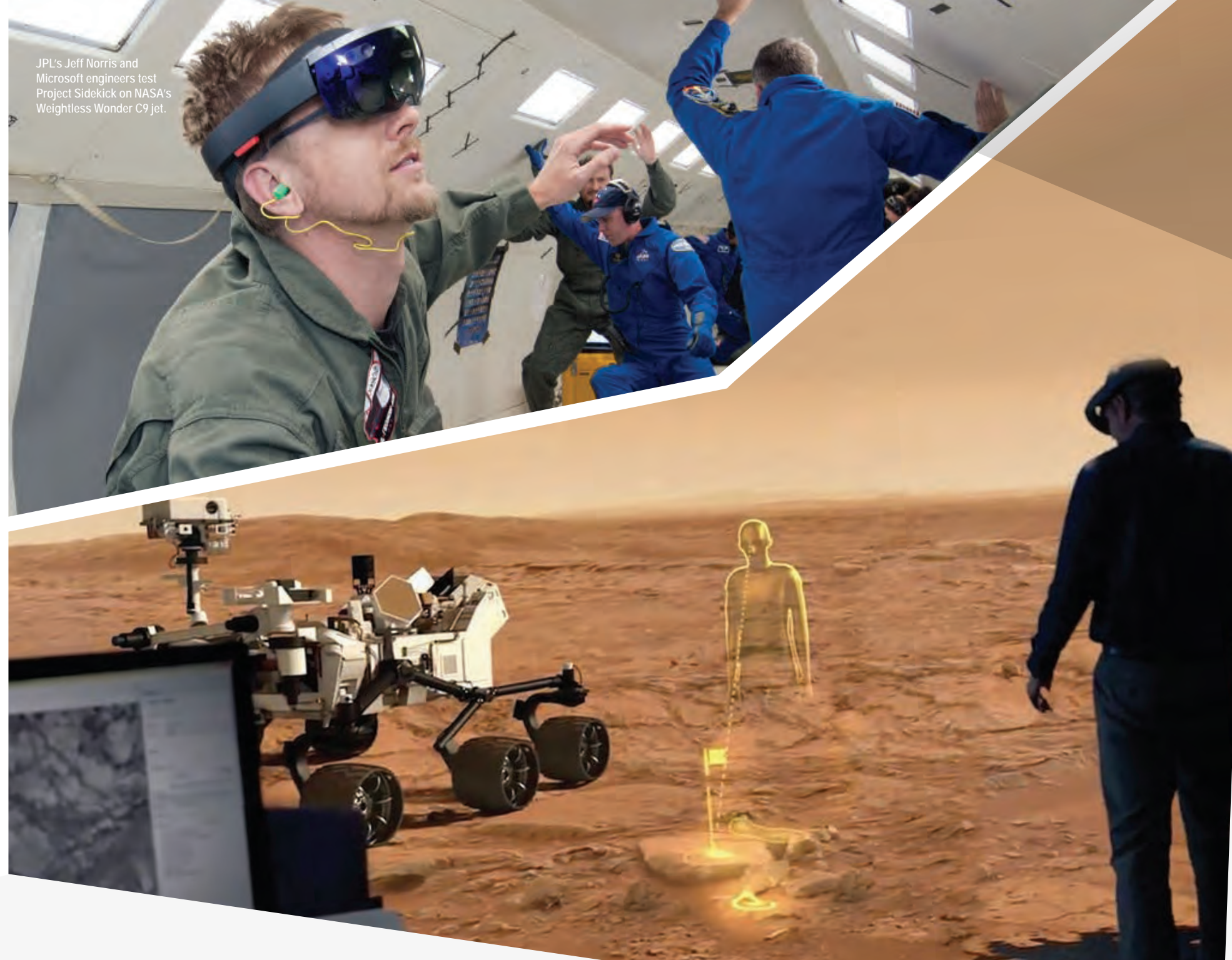
[A-B] Screen views from OnSight, a software tool developed by NASA's Jet Propulsion Laboratory in collaboration with Microsoft. OnSight uses real Mars rover data to create 3-D simulations of the Martian environment where mission scientists can "meet" to discuss rover operations and do science planning. The tool provides access to scientists and engineers looking to interact with Mars in a more natural, human way. [C] Astronaut Scott Kelly used Sidekick to make the first Skype call from space. By connecting astronauts to experts on the ground, mixed reality could be transformational for scientific and engineering efforts in space.
