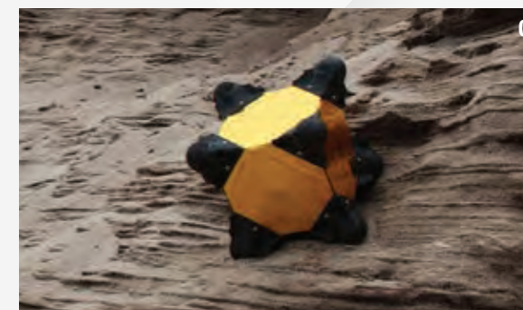
[Left] JPL Principal Investigator Issa Nesnas and Stanford engineers conducting hopping experiments aboard NASA's C-9 parabolic aircraft. [A] The basic concept is a cube with spikes that moves by spinning and braking mutually-orthogonal internal flywheels. [image credit] Stanford. [B] Hedgehog robot aboard NASA's C-9 aircraft lifting vertically off granular material (garnet sand). [C] The Stanford Hedgehog hopping/tumbling robot prototype on rugged terrain. [image credit] Prof. Marco Pavone, Stanford University.
