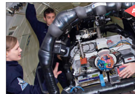
A A JPL team successfully tests magnetic flux pinning aboard a microgravity simulation flight. B The Orbiting Sample is positioned to be magnetically captured by the superconductors aboard the Earth Return Vehicle. C Principal Investigator Laura Jones-Wilson demonstrates magnetic flux pinning.
