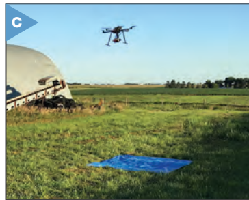
A — Researchers adjust instrumentation before deployment over a crop field. B — The MAV is adapted from commercially available quadcopters. Once it reaches the end of a flight, or is nearing battery depletion, it lands at a charging station autonomously. C — A MAV takes flight to complete its autonomous circuit of crops. Information is stored onboard for downloading at the completion of its flight. D — From high in the air, the MAV autonomously gathers data about plant hydration from the crops below.
