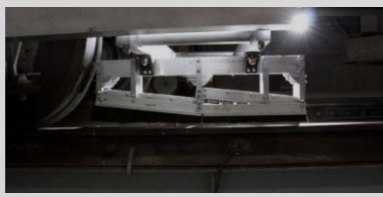
Passive-only rail inspection prototype mounted on DOTX216 car during field test at TTC.
