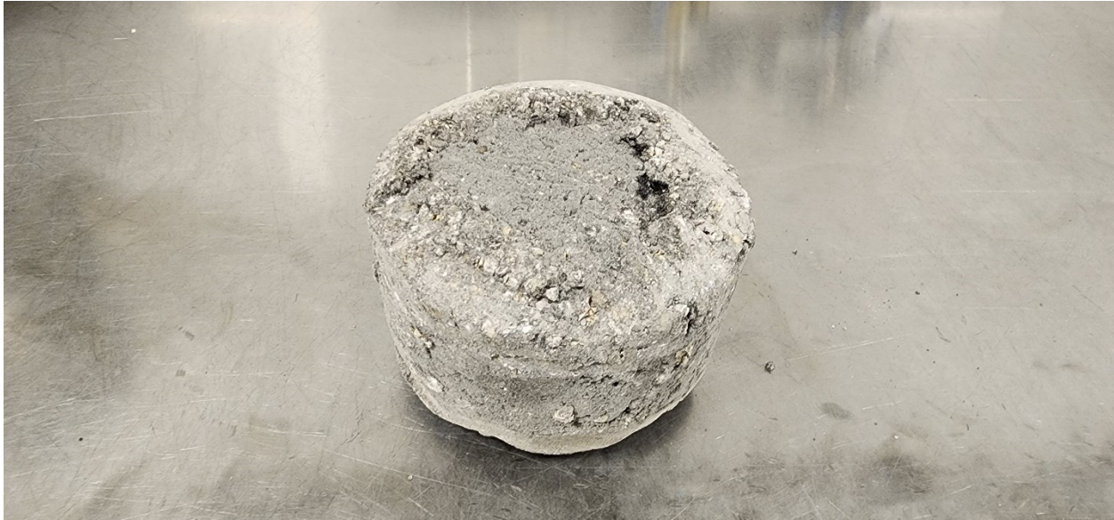
Figure 24. Specimen after Cantabro Test.
