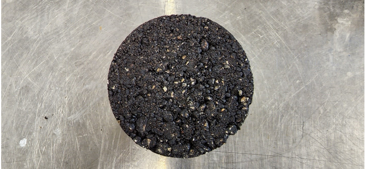
Figure 22. Specimen after IDEAL-RT Test.
