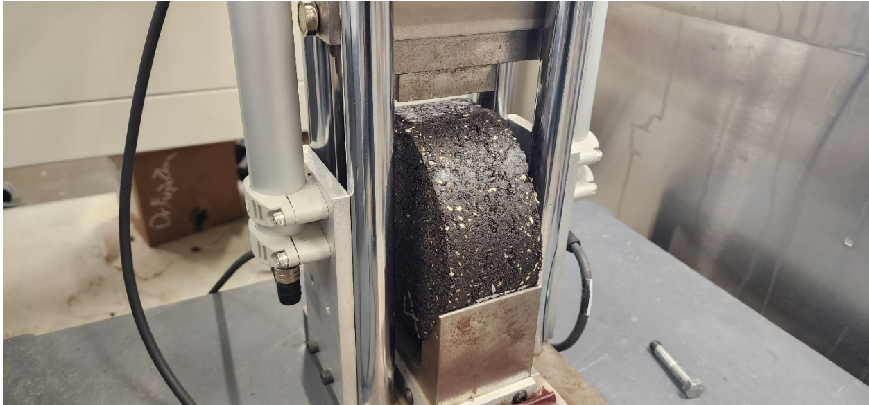
Figure 21. Setup of IDEAL-RT Test.
