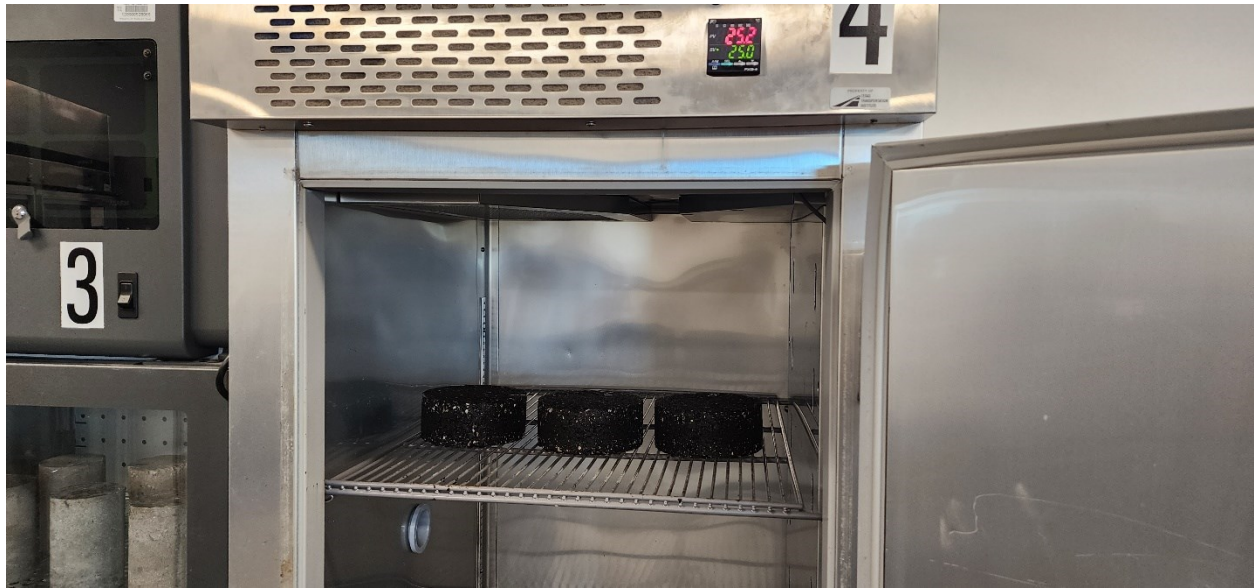
Figure 27. Conditioning of IDEAL-CT Specimens.
