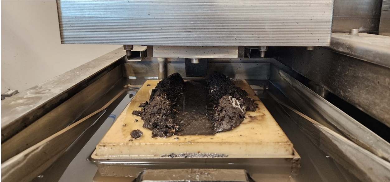
Figure 19. Rut Depth after 1014 Load Passes.
