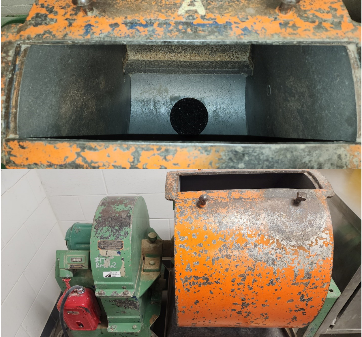
Figure 23. Setup of Cantabro Test.
