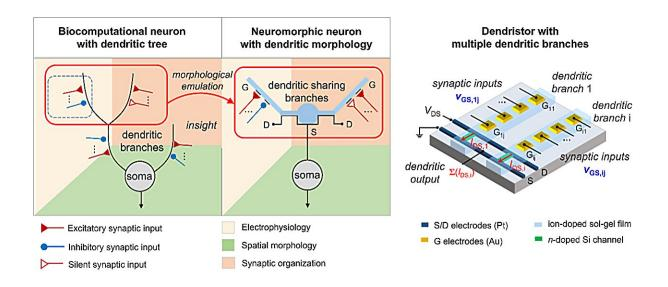
The Dendristor mimicking dendritic morphology. Credit: Adapted from *Nature Electronics* (2024). DOI: 10.1038/s41928-024-01171-7
