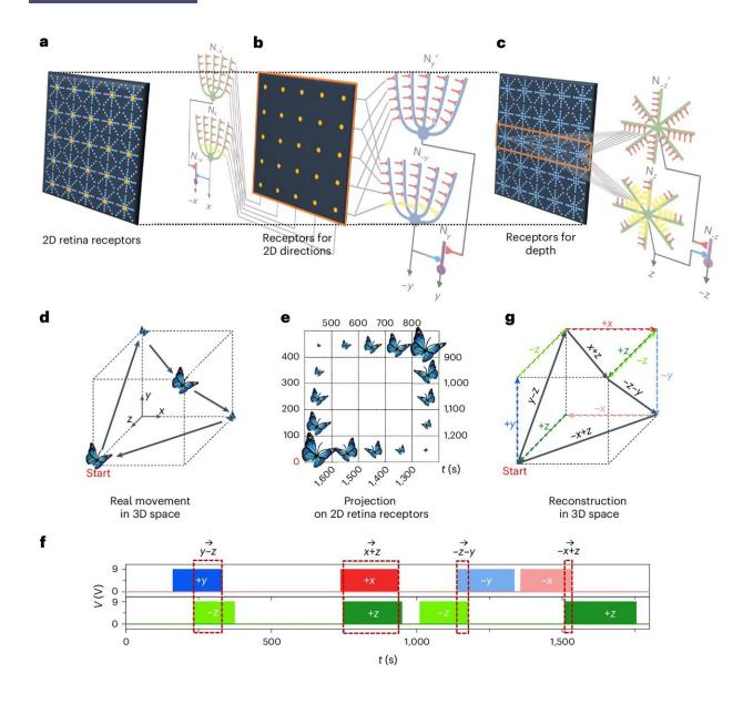
3D visual motion perception of dendritic network neural circuits. Credit: *Nature Electronics* (2024). DOI: 10.1038/s41928-024-01171-7
