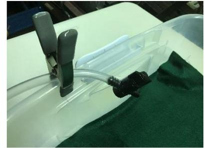
Step 17: Place the vinyl tubing extending from the discharge end of the container (elbow) into the small Tupperware or water storage container and secure it with a spring clamp.
