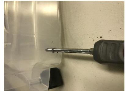
Step 3: Use a pre-heated glue gun to melt and widen the hole so that it is just large enough to push through the threaded lamp nipple. This should be a tight fit.
