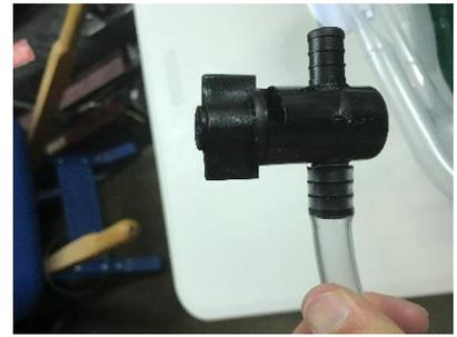
Step 16: Attach the vinyl tubing to the upstream end of the container (opposite end of the threaded lamp nipple outlet) using a spring clamp.
