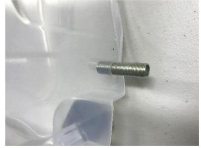
Step 6: Add rubber washer to the inside and outside part of the threaded lamp nipple and make sure it fits firmly against the container.
