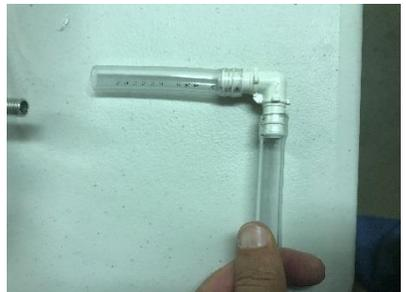
Step 10: Attach the short end of the tubing to the threaded lamp nipple as shown and secure with a zip tie. Make sure to slide the tubing all the way up the threads. **HINT: Slightly heating the tubing with a hot hair drier or other means can help it to expand, making this task a little easier.**
