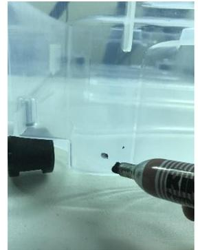
Step 2: Use a standard Phillips head screwdriver to melt a small hole through the container at the mark. Use a lighter to heat the tip of the screwdriver so that it will melt the plastic.
