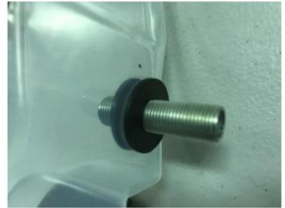
Step 7: Screw on the brass lock nuts and hand-tighten as much as is possible. Over-tightening the lock nut by using pliers can damage the container.
