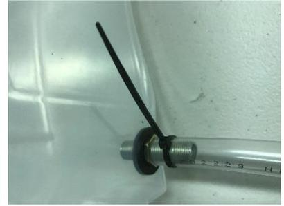
Step 11: Cut a small square piece of nylon window screen. Fold the piece over the inside part of the threaded lamp nipple and secure with a zip tie to prevent large particles from getting through and clogging the pump.
