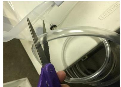
Step 9: From the 5-foot section of clear vinyl tubing, cut off a 3-inch piece of tubing, and connect the elbow attaching both pieces as shown.
