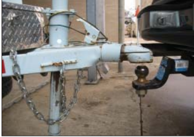
Figure 1. Align trailer hitch over ball on vehicle
