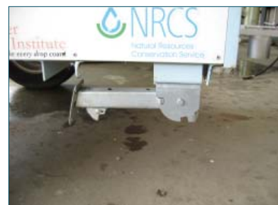
Figure 8. Rear jack stands in an up position
