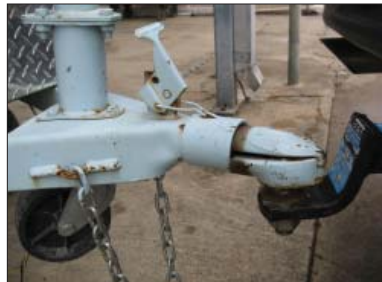
Figure 2. Lower trailer hitch on ball
