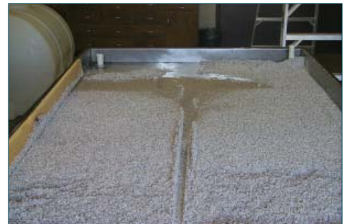
Reservoir created with a channel sloping down the trailer.
