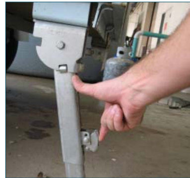
Figure 9. Rear jack stand in a down position
