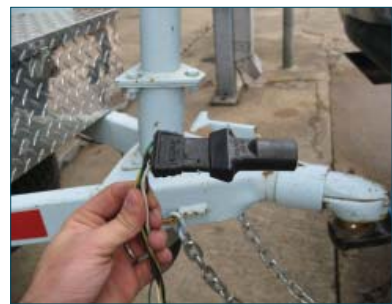
Figure 7. Light wiring harness adapter
