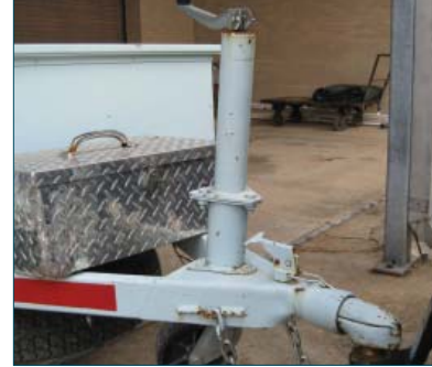
Figure 5. Jack in an up position
