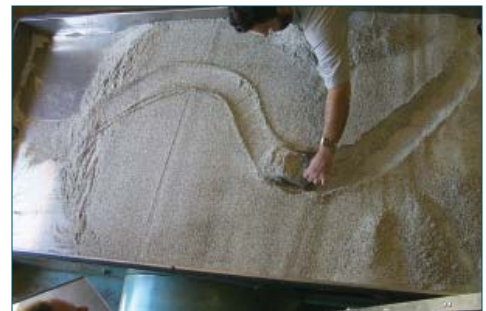
Dig out the channel with a scoop.
