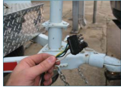
Figure 6. Standard light wiring harness
