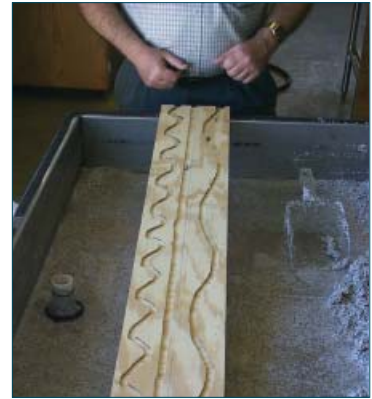
The stream channel board has three grooves to show the difference in water flow in straight and curvy streams.
