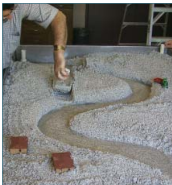
Cut through a bend to straighten the stream.
