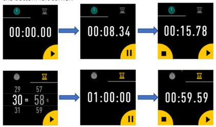
For timer function, maximum countdown time is 120min 59sec. After starting the countdown, the down-counting time is displayed as format HH:MM:SS.
