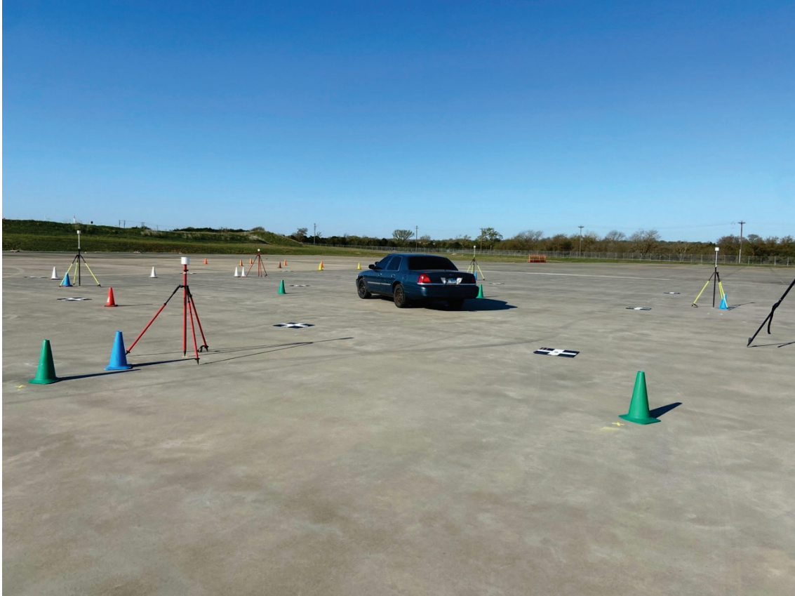
Figure 232. TLS Target Setup on Instrument Points and an Additional Target Tie Point.
