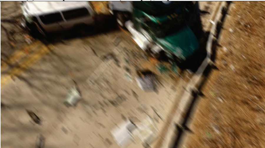
Figure 156. Image Quality Degradation for Different Exposure Times and UAS Speeds.
