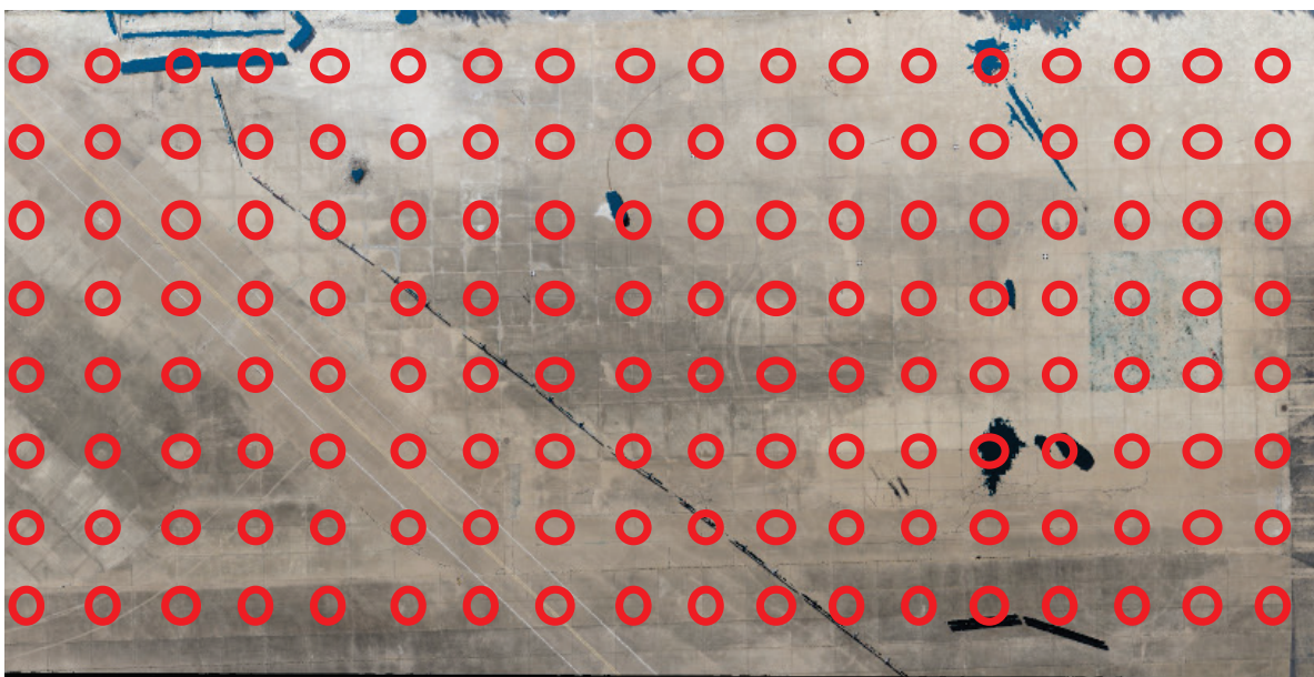
Figure 202. Circular Patches for Computing Surface Roughness (not to scale).
