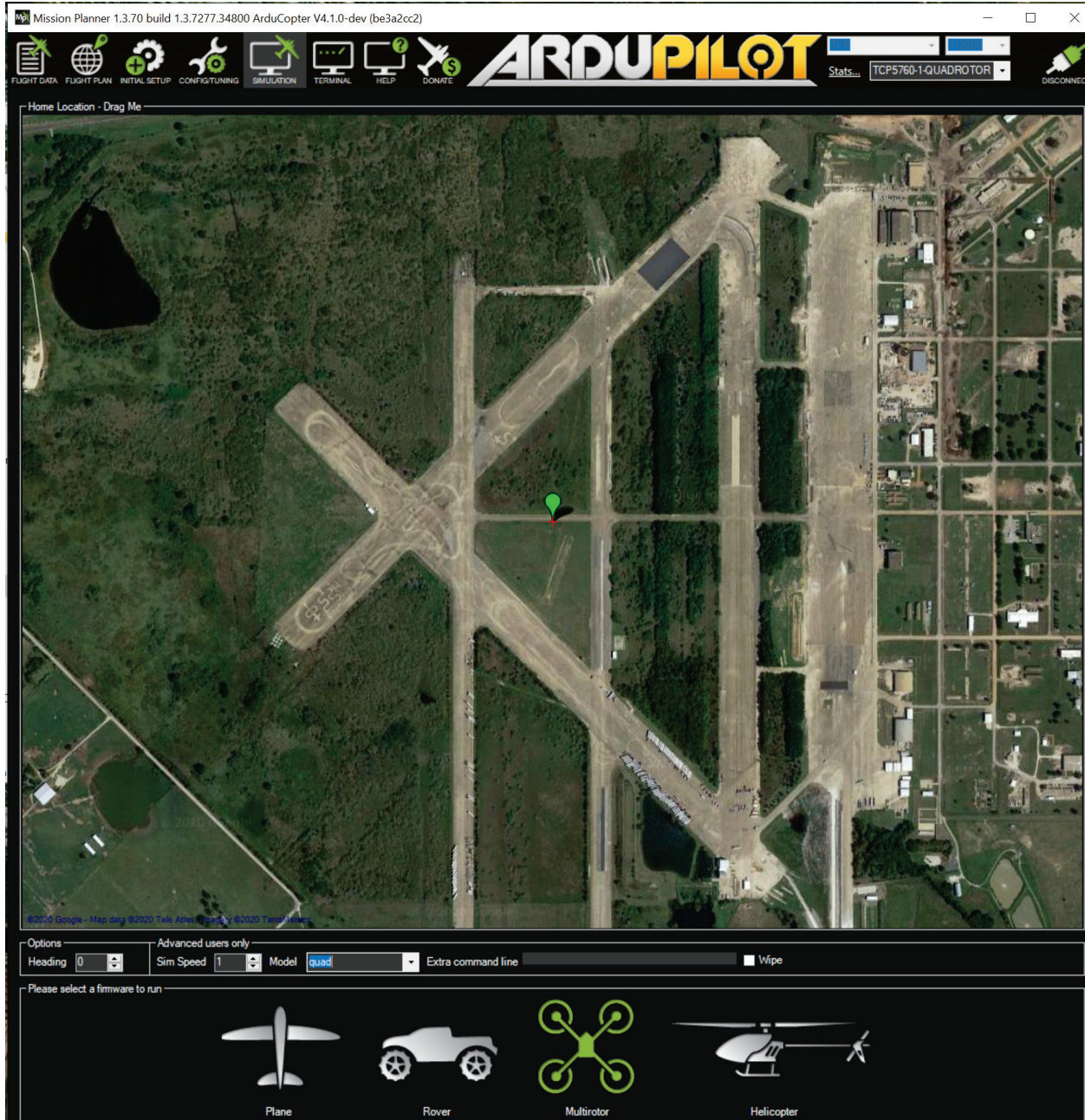
Figure 39. Screen in Mission Planner Where Simulation Starts and Craft Type Is Selected.
