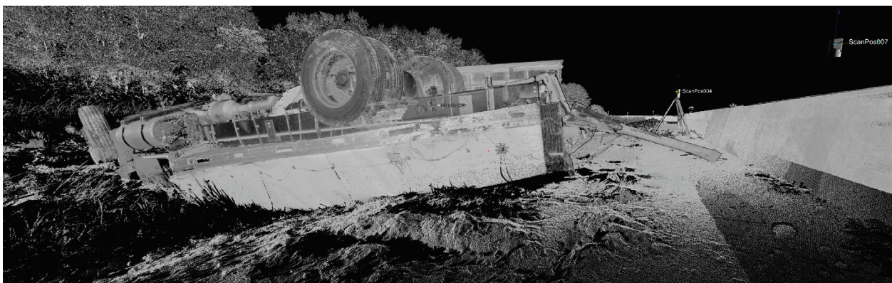
Figure 214. Oblique View of TLS Point Cloud of Crashed Vehicle.
