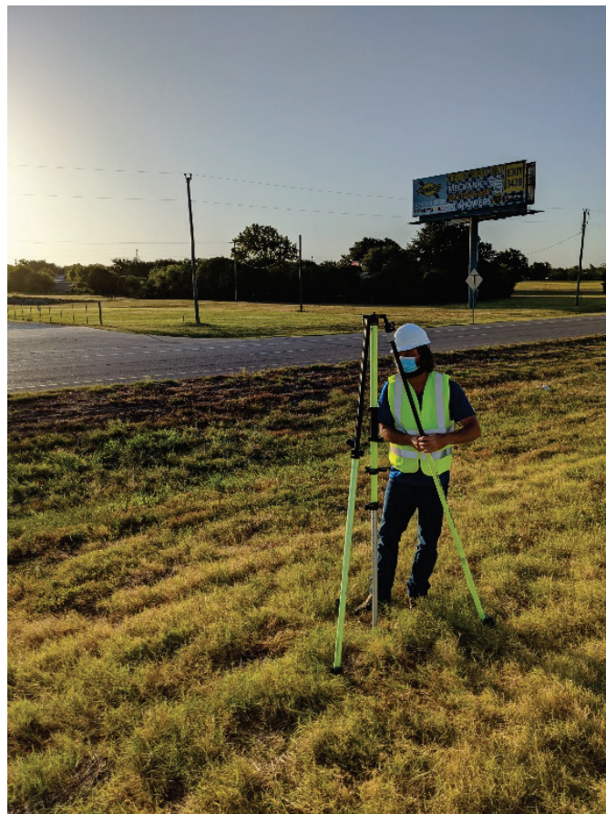
Figure 179. Static Observation GNSS Receiver Being Set Up.
