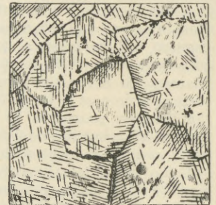
FIG. 2.—Pearlite with ferrite. (Sorby.) The polygons are pearlite; the network is ferrite.
