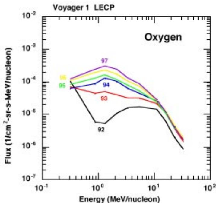
The LECP instrument uses very thin silicon solid state detectors (the thinnest is only 2 microns thick, about 1/30 the thickness of a human hair) to measure the oxygen flux down to 200 keV/nucleon.
