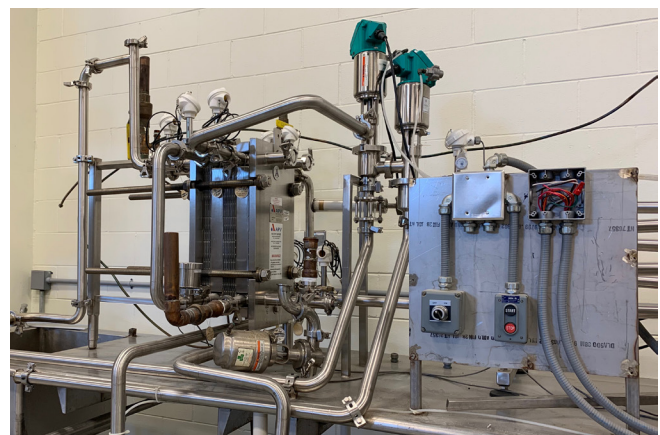
Figure 2. This is an example of a heat exchanger that a liquid would flow through prior to packaging. (Photo courtesy of Renee Boyer.)
