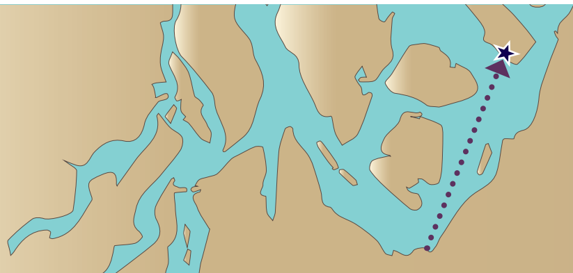
Maximum fetch (arrow) is the longest distance across open water to a site (star).
