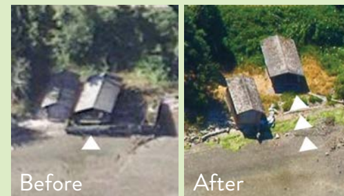
The building on the right was moved back and the bulkhead removed.
