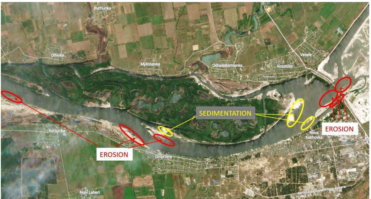
Figure 12. Localities with major erosion and sedimentation at the dam breach site and close downstream, identified on satellite images Sentinel-2 (Source: Sentinel-hub EO-Browser3 2023)
