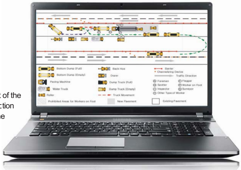
The above ITCP diagram includes a legend and notes (Sources: ARTBA and FOF Communications; clipboard drawing below: FOF).
