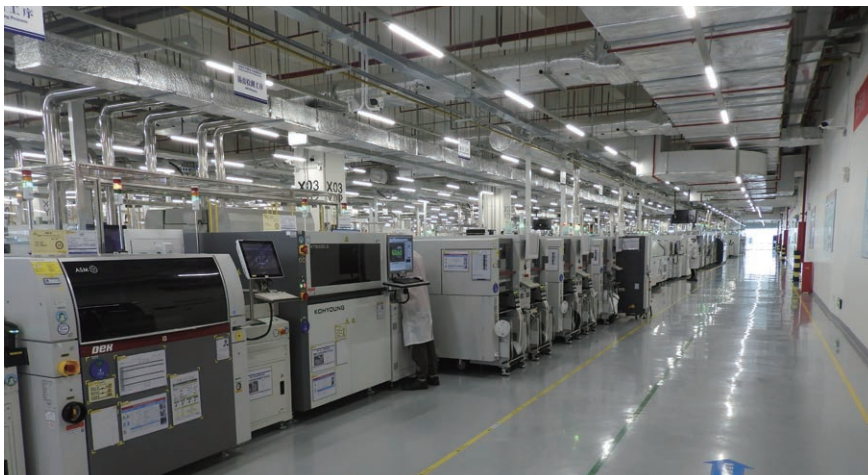
One-piece flow: Automated, lean production line of on-board chargers (OBCs) for intelligent electric power
