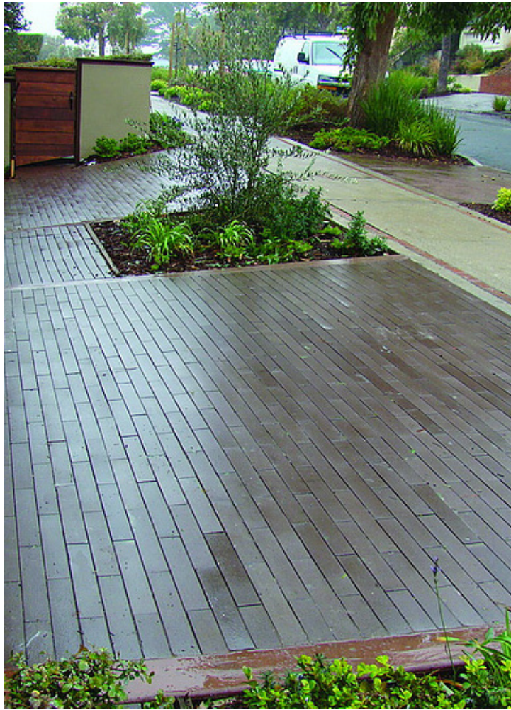
STEPSTONE - NARROW MODULAR PAVER (SPECIALTY PAVING)
