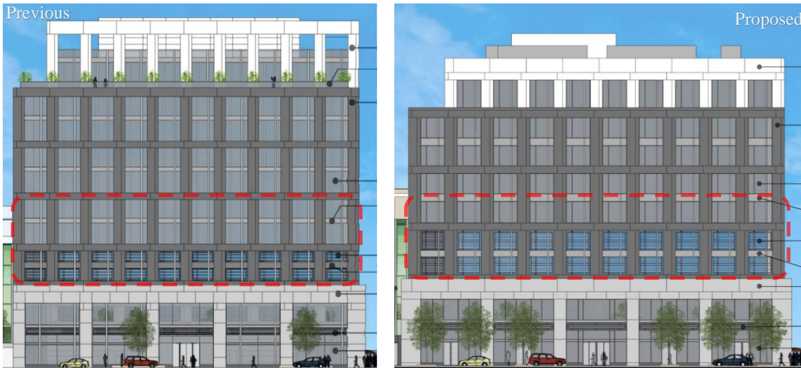
Figure 7: The manipulation of the ceiling heights and the elimination of two levels on the building have significantly altered the proportions and scale of the North Tower.
