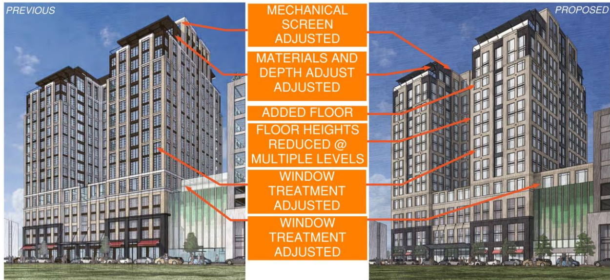
Figure 6: Applicant proposes the following changes to the South Tower, as viewed from the Northeast on future John Carlyle Street.
