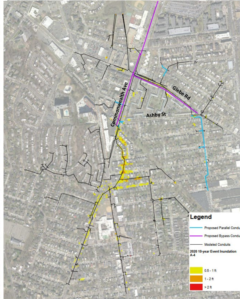
Figure 16. Current (Year 2020) 10-Year Storm Predicted Flood Inundation under Current Conditions and Preferred Alternatives
