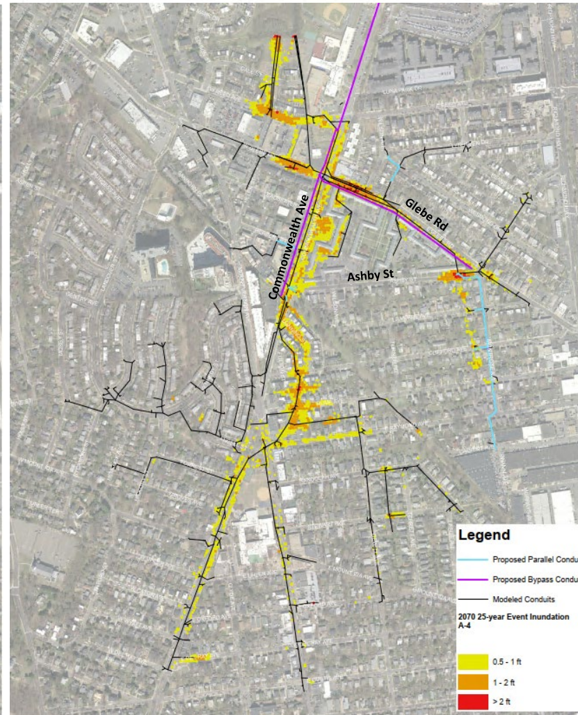
Figure 17. Future (Year 2070) 25-Year Storm Predicted Flood Inundation under Current Conditions and Preferred Alternatives
