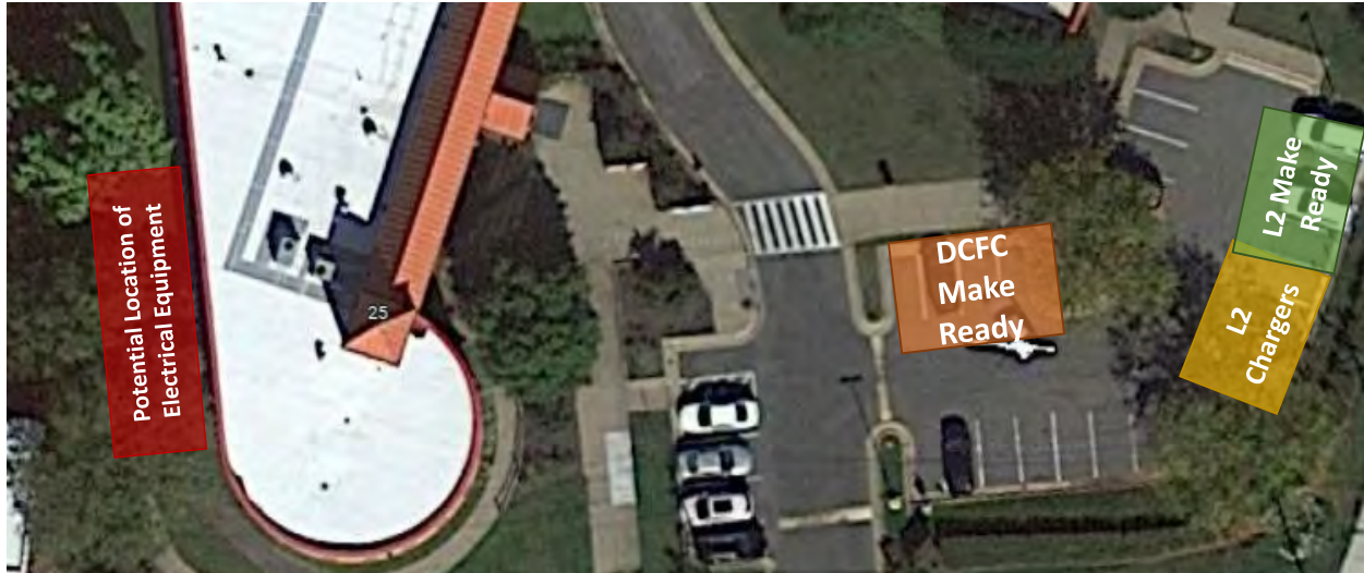
Figure 15. Proposed Leonard “Chick” Armstrong Recreation Center Charging Installation Site Plan (Not to scale)
