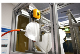
Non-destructive testing for medical PPE suit to verify its readiness
