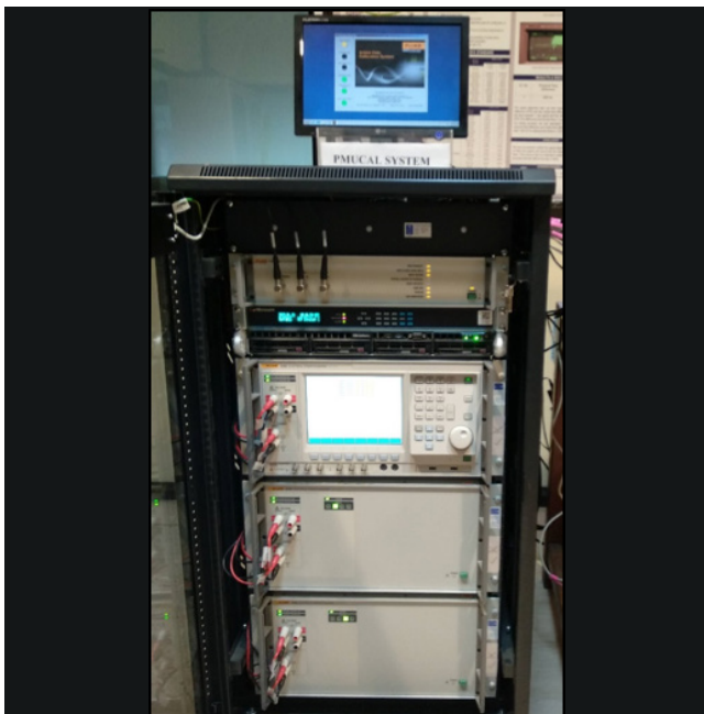
Fig.1: CSIR-NPLI Phasor Measurement Unit Calibration System (PMU-CAL)
