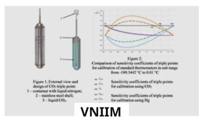
Triple point of carbon dioxide to replace fixed point of mercury
